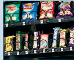
The well proven, dual spiral vending system fitted to snack and food trays is reliable, easy to adjust and suitable for a wide variety of products. The spirals gently but firmly support the products and smoothly move each item forward to the vend position.
