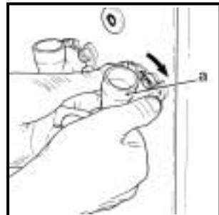
5. Refit the whipper bases (a). Rotate the base anti-clockwise to lock into position as shown.
