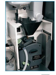
Evolution machines fitted with either the CoEx® or double freshbrew brewer must be fitted with a water hardness reducing filter. Crane Merchandising Systems recommend and supply the Brita AquaQuell compact water filter.
